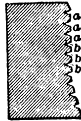
Fig. 6. Finishing end of the die.
