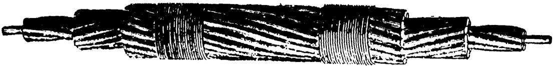
FIG. 179.—M. Arnodin's alternately twisted cable, one-third of the natural size.
