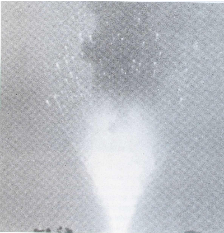
Figure 4–22(a). Propellant chunks ejected in 260" motor test.
